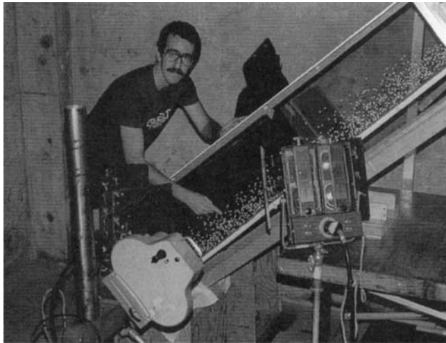
FIGURE 1. A typical disperse flow in the 3.7 m long, 0.5 m deep and 6.7 mm wide experimental chute. Plastic spheres 6 mm in diameter contained in a hopper above and behind the upper end of the apparatus feed onto a gently inclined tray, organizing into a single layer that spills into the head of the chute, where they form an essentially two-dimensional grain flow. The bed for the flows is the light-coloured strip inside the chute, which can be independently adjusted through a small range of angles to fine-tune the inclination. The flows approach a nominally steady, uniform condition rapidly, typically in 10–15 flow depths. A 16 mm camera operating at about 1440 frames per second or 60 times the normal projection rate documents particle motion; the centre of the camera field is about 70 cm upstream of the chute outlet.
